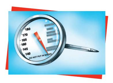
■ **Dial instant-read**—not designed to stay in the food during cooking. Insert probe the full length of the sensing area, usually 2 to 2 1/2 inches. If measuring the temperature of a thin food, such as a hamburger patty or boneless chicken breast, insert probe sideways with the sensing device in the center. About 15 to 20 seconds are required for the temperature to be accurately displayed.
